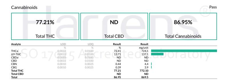
1 Unit = g. 1g. Determination of Cannabinoids by HPLC, HL223 Total THC = THCa \*  $0.877 + \Delta 9$ -THC Total CBD = CBDa \* 0.877 + CBDND = Not Detected; NR = Not Reported; LOD = Limit of Detection; The reported result is based on a sample weight with the applicable moisture content for that sample; Unless otherwise stated all quality control samples performed within specifications established by the Laboratory. HL105.10-01
